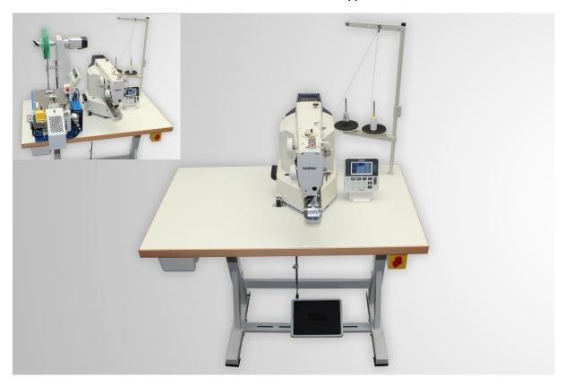
This automatic bartacker can be placed directly next to the lifttape cutter to ensure a continuous and smooth production flow.
